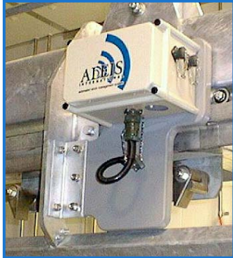
Model 3501 Aleis HookTraka System Installed at selected locations on abattoir floor. Automatically reads individual hooks.
