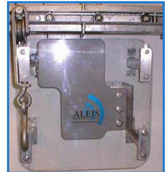
Model 3503 Aleis Hook Room System Confirms hook status prior to going on kill floor.
