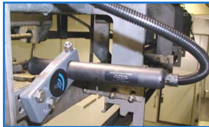
Model 3502 Aleis HookTraka Wand Installed at selected locations on abattoir floor. Automatically reads individual hooks.
